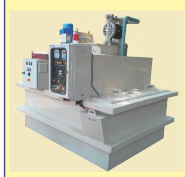
The fluxing bath is being polluted by acid residues and above all by dissolved iron. Consequently it makes the quality of the galvanizing process worse; moreover iron being entered by a polluted fluxing flow into the galvanizing bath binds itself with zinc and precipitates to the bottom, thus increasing dross.
