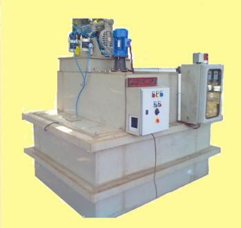
View of a continuous flux regeneration system
