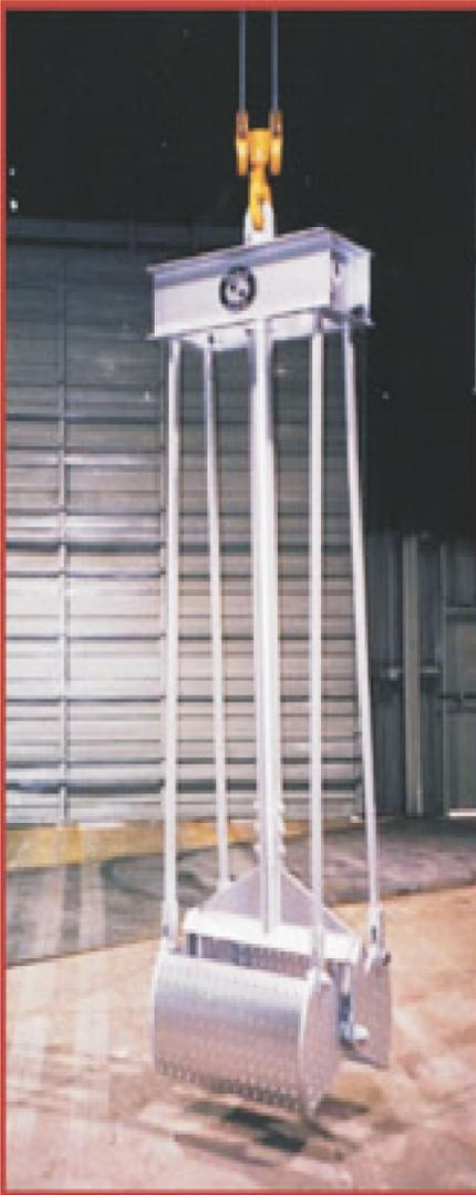
The dross grab is fabricated in stabilized stainless steel sized to suit your galvanizing kettle dimensions. The two grab flaps are perforated with suitable sized holes to allow free molten zinc to run back into the bath.
